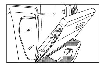
Open the tailgate by pulling up on the outside handle while pulling the tailgate down.
